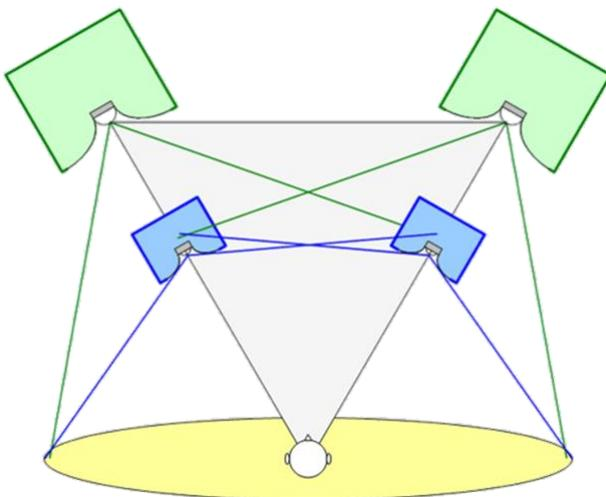
The longer distance between a larger monitor and the listening position brings in more of the character of the room, i.e. modes and reflections. To control the impact of these influences on the perceived sound quality, the dispersion on larger monitors should be narrower.
