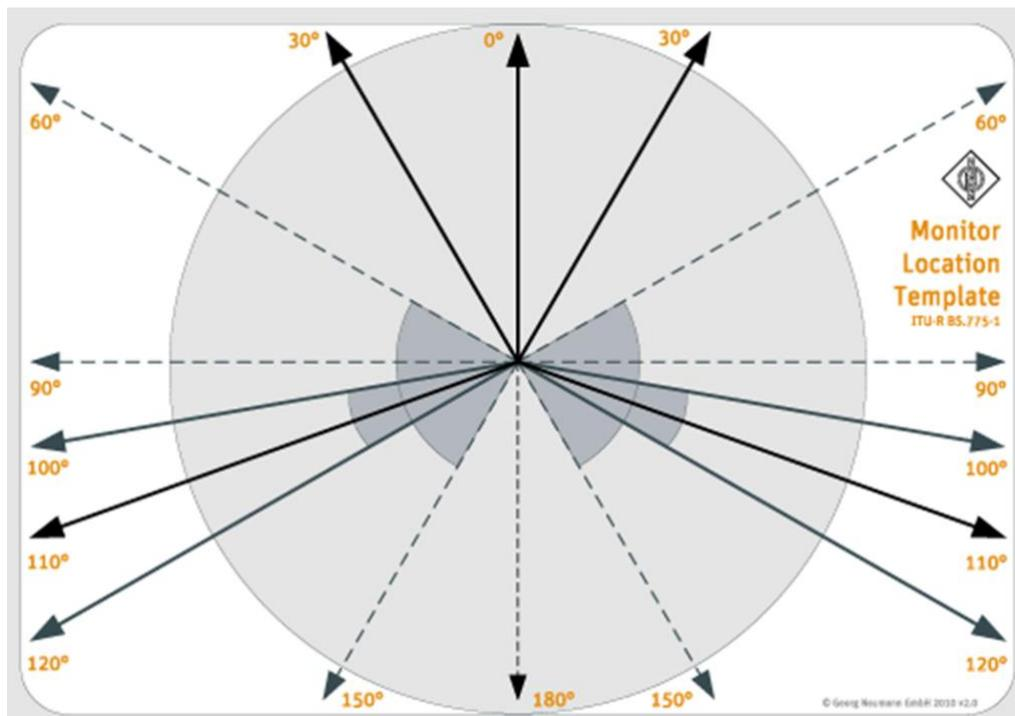
Use this template to help position the loudspeakers’ acoustical axis at the correct position:
