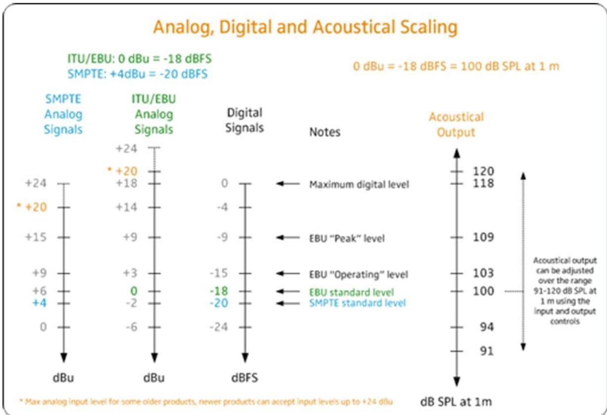
Next the signal is aligned to an acoustical output of the loudspeaker that results in the required level at the listening position. Here is the complete process:
